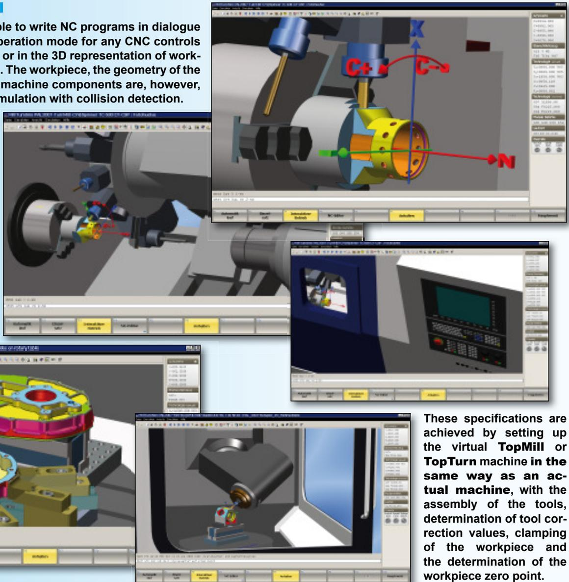
These specifications are achieved by setting up the virtual **TopMill** or **TopTurn** machine in the same way as an actual machine, with the assembly of the tools, determination of tool correction values, clamping of the workpiece and the determination of the workpiece zero point.
