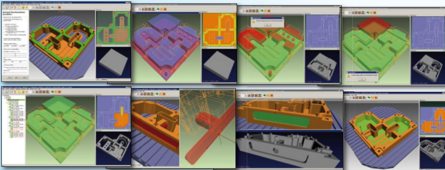
**TopCAM3D** is a machining plane oriented 3D milling programming system with automatic machining feature recognition for classic, multi-sided machining of usually complex machine parts with 5-axes machining centers.
